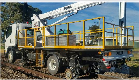
Available in over-center, air suspended, or pivoting axle configurations to suit the RRV application
